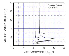
Fig 5. Saturation Voltage vs. V<sub>GE</sub>
