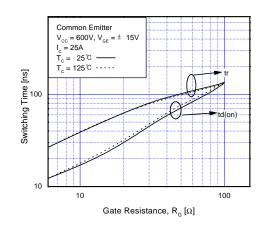
Fig 8. Turn-On Characteristics vs.
