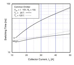
Fig 11. Turn-On Characteristics vs. Collector Current
