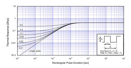
Fig 17. Transient Thermal Impedance of IGBT
