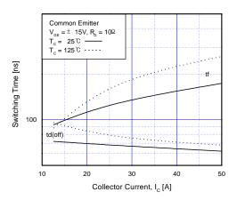
Fig 12. Turn-Off Characteristics vs. Collector Current
