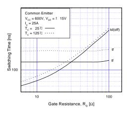
Fig 9. Turn-Off Characteristics vs.
