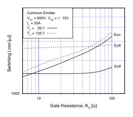
Fig 10. Switching Loss vs. Gate Resistance
