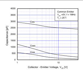
Fig 7. Capacitance Characteristics
